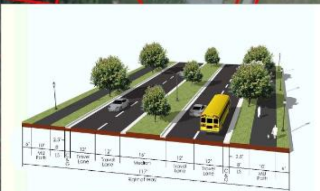
Typical Four-Lane Cross Section ASHLAND ROAD
