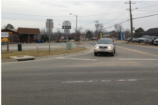
Photograph 4: Looking at Eastbound Approach Stop Bar Placement
